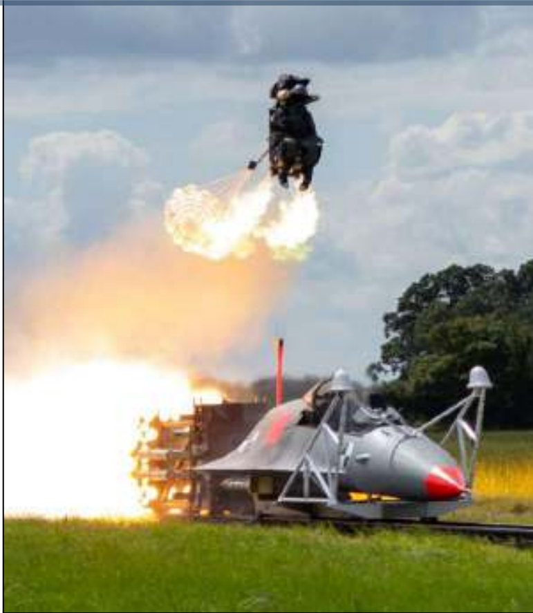
© US18E ejection test at MBA test facility
